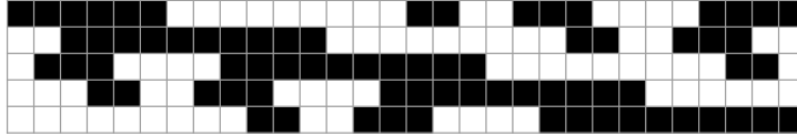
Figure 1: A 5-digit single-track Gray code with period 30 where every component sequence is a cyclic shift of 111111111100000000011001110000.
